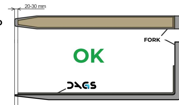
Once DAGS has been fitted, correct positioning must be determined before using it. The magnetic device must be firmly secured without protruding from the fork contour.
